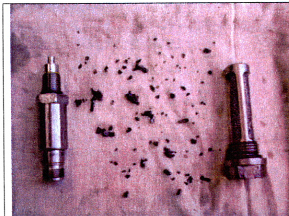
L&S filter screen contamination
